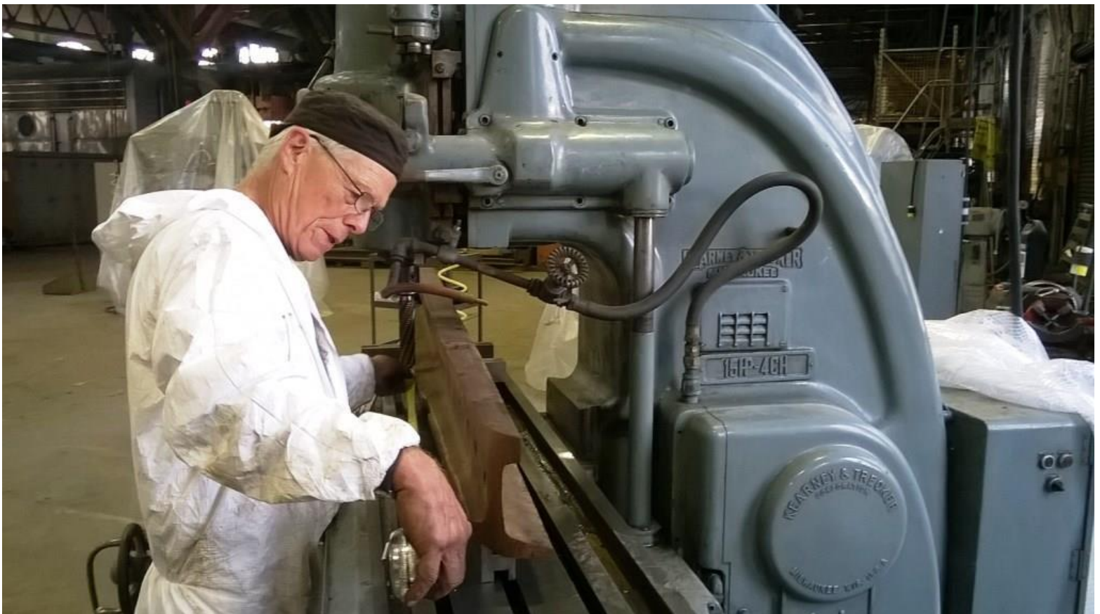
Jim Bays milling the wing-rail for the frog at Switch 19
