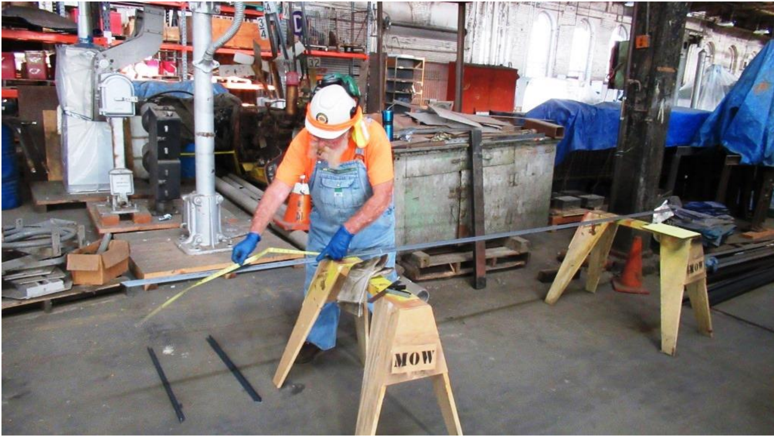
Pat measures a strip of steel for use in the anti-vandalism shields for the ride-on spiker
