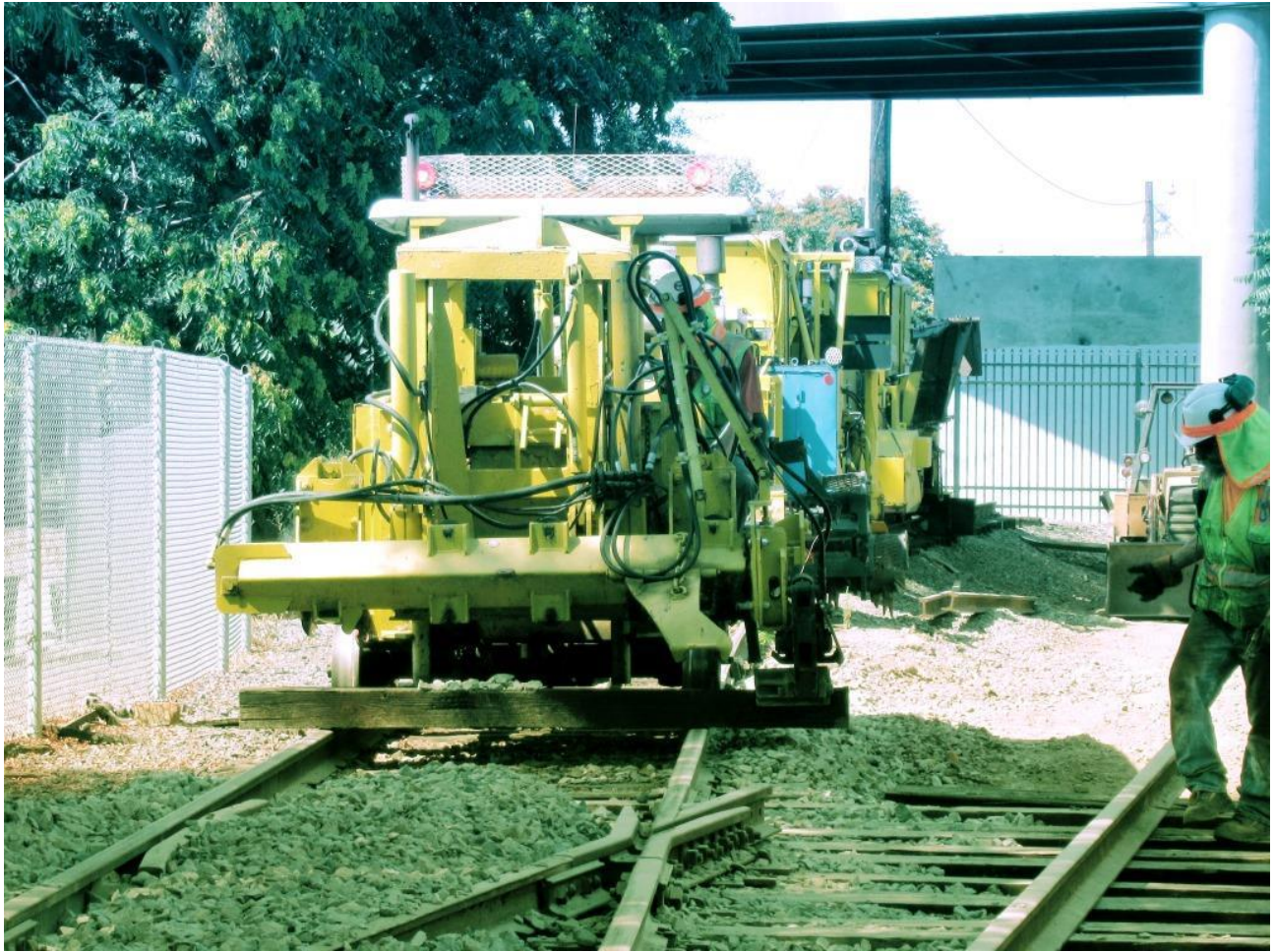
Here's the easier way. Use the Jackson 125 as a rock-plow
