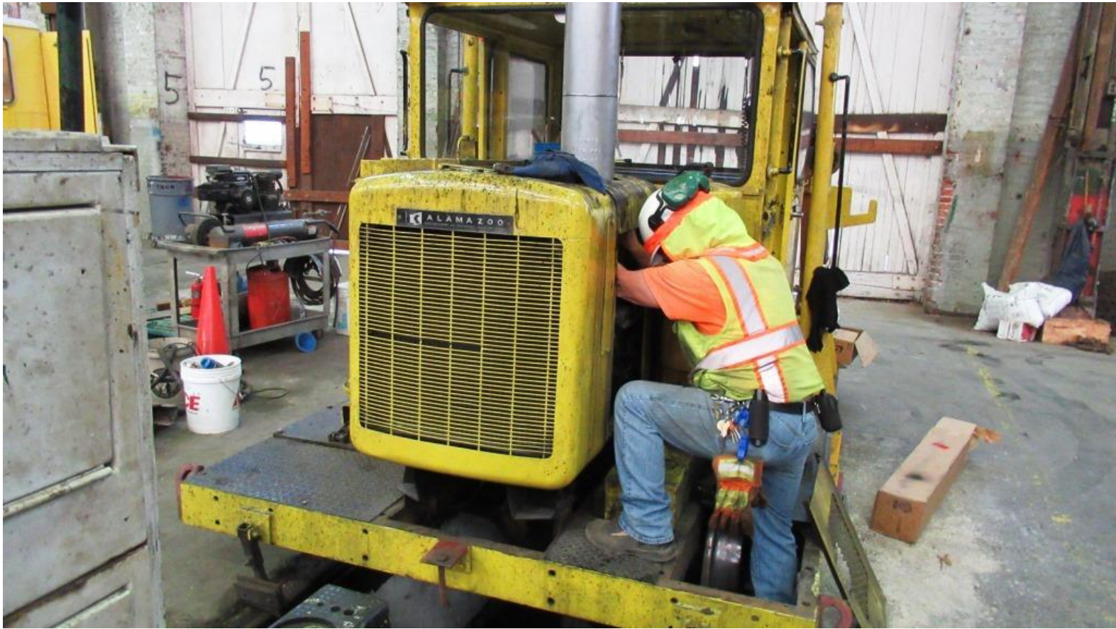
Joe installs the new muffler on the Kalamazoo
